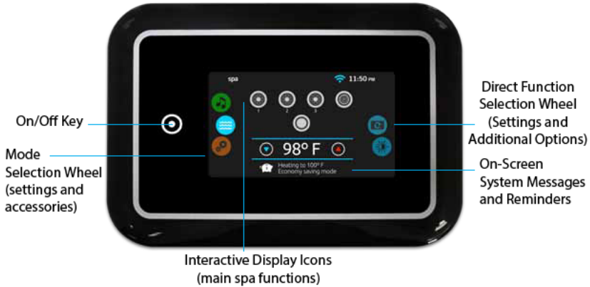
in.k1000 Control Panel
