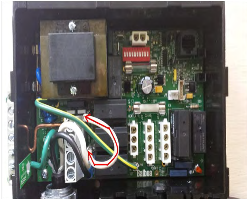
FIGURE 3—Remove Jumper from J28 and J57
